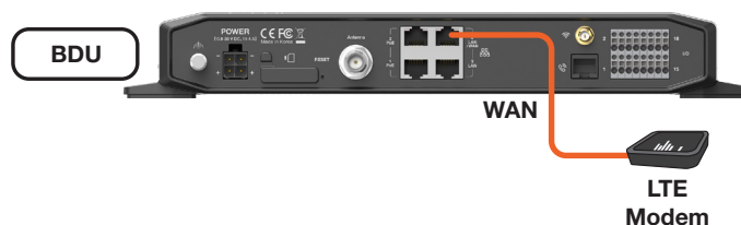
Figure 38: BDU to Device Cable Connection using WAN Port
